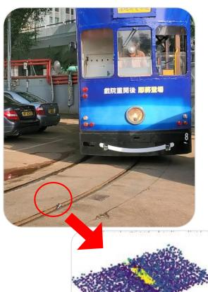
**Tramway Track Small / Foreign Object Detection System**
