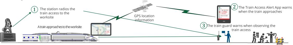
The station radios the location of worksite to the train driver The Train Access Alert App also warns the location
